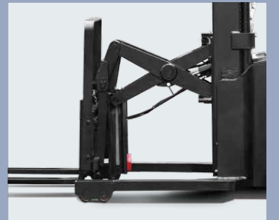
Forks move forward by the scissor structure
